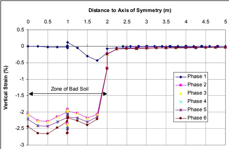
Figure 5: Vertical strain at the top of the subgrade.
