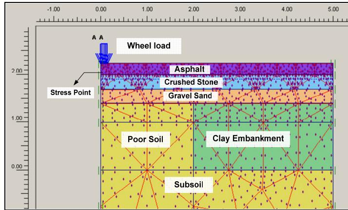
Figure 3: Axi-symmetric model for inhomogeneous soil layer.
