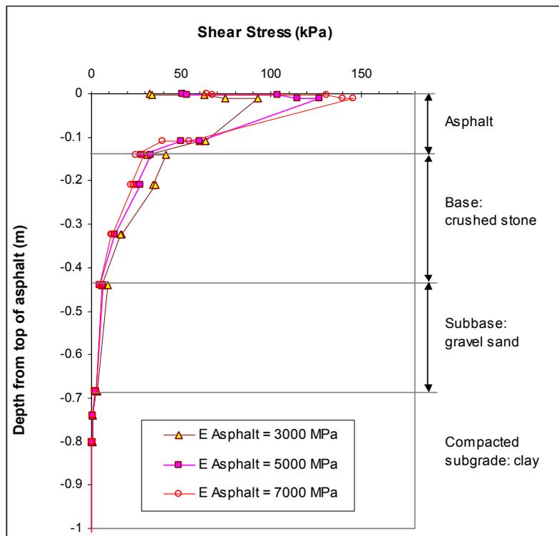
Figure 11: Shear stress distribution for various asphalt stiffnesses.
