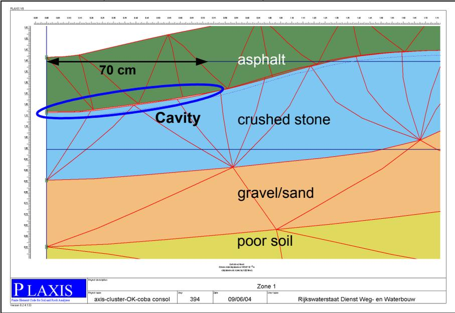
Figure 6: Deformed mesh in phase 2: consolidation 500 days.
