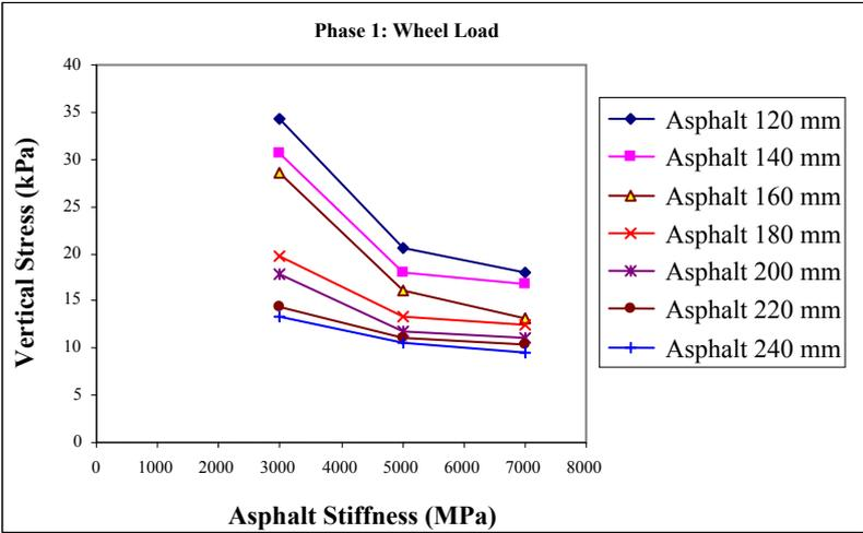
Figure 9: Vertical stress on top of subgrade as a function of asphalt stiffness and thickness.
